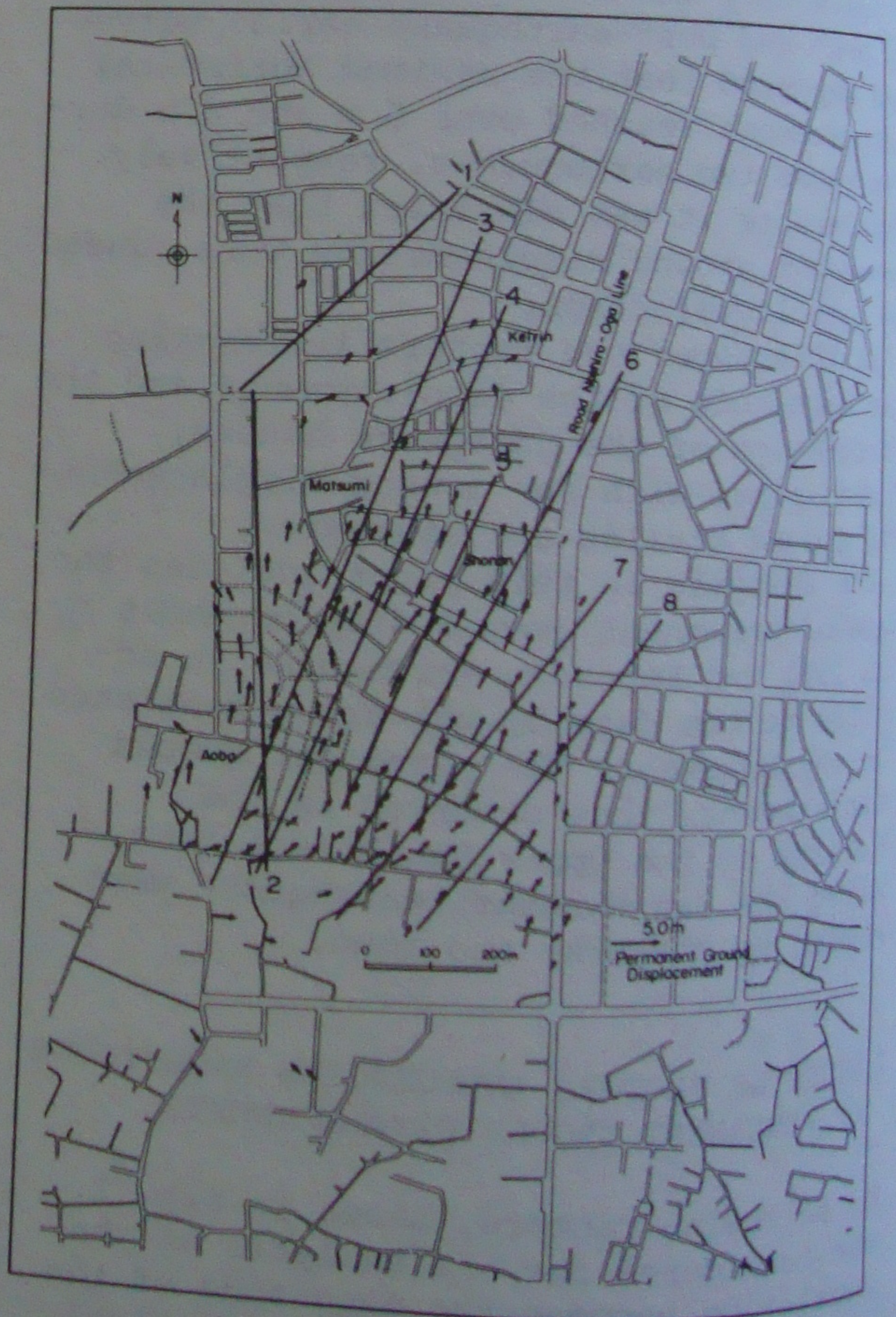
Fig. 2 Sector lines for the survey of soil condition in northern part of Noshiro City
